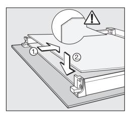
Replace the second of the middle panes. Make sure the cut-off corner is positioned at the top left hand side.
